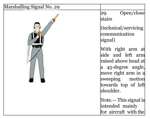
(1) Signals from the pilot of an aircraft to a signalman. The pilot-inocommand or co-pilot shall use the following signals when communicating with signalman:
